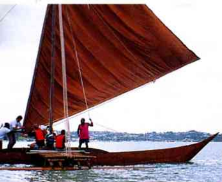
Mast is upright and sail is passed round on the lee side.
