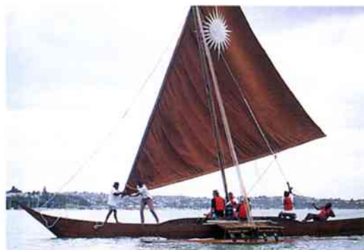
... and carried aft, while the crew at the stern pull on the stay to cant the mast upright
