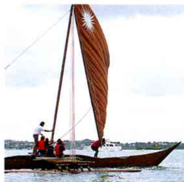
As sail moves on, the mast cants through further.
