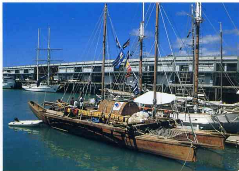
Cook Island double canoe Te Au O Tonga. 70' replica built in ply and epoxy.
