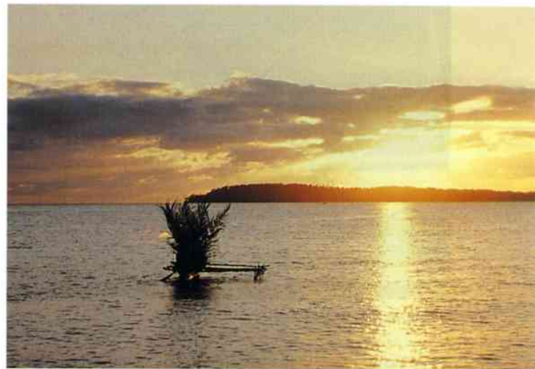
This canoe is being sailed by the most basic of sails, ie four palm leaves lashed together to make a downwind rig.
