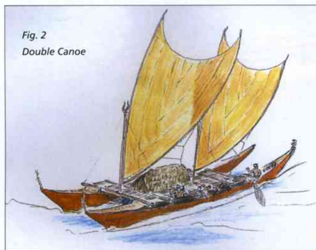
Cook Island double canoe Te Au O Tonga. 70' replica built in ply and epoxy.
